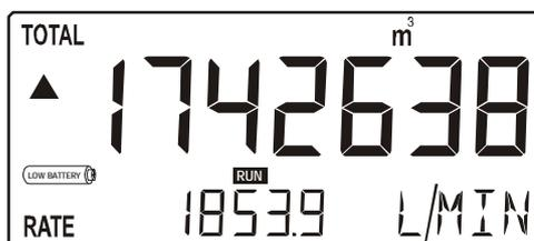
*Fig. 4: Example of low-battery alarm.*
