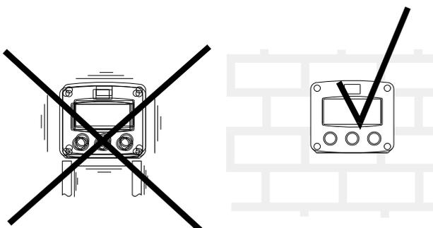
Mount the F110-P on a solid structure to avoid vibrations.
