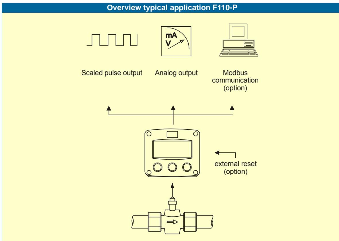
Fig. 1: Typical application for the F110-P.
