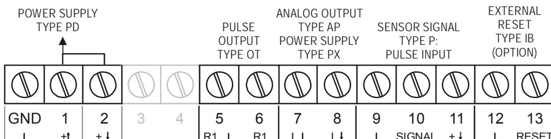
Fig. 12: Overview terminal connectors XI - Intrinsically Safe applications.
