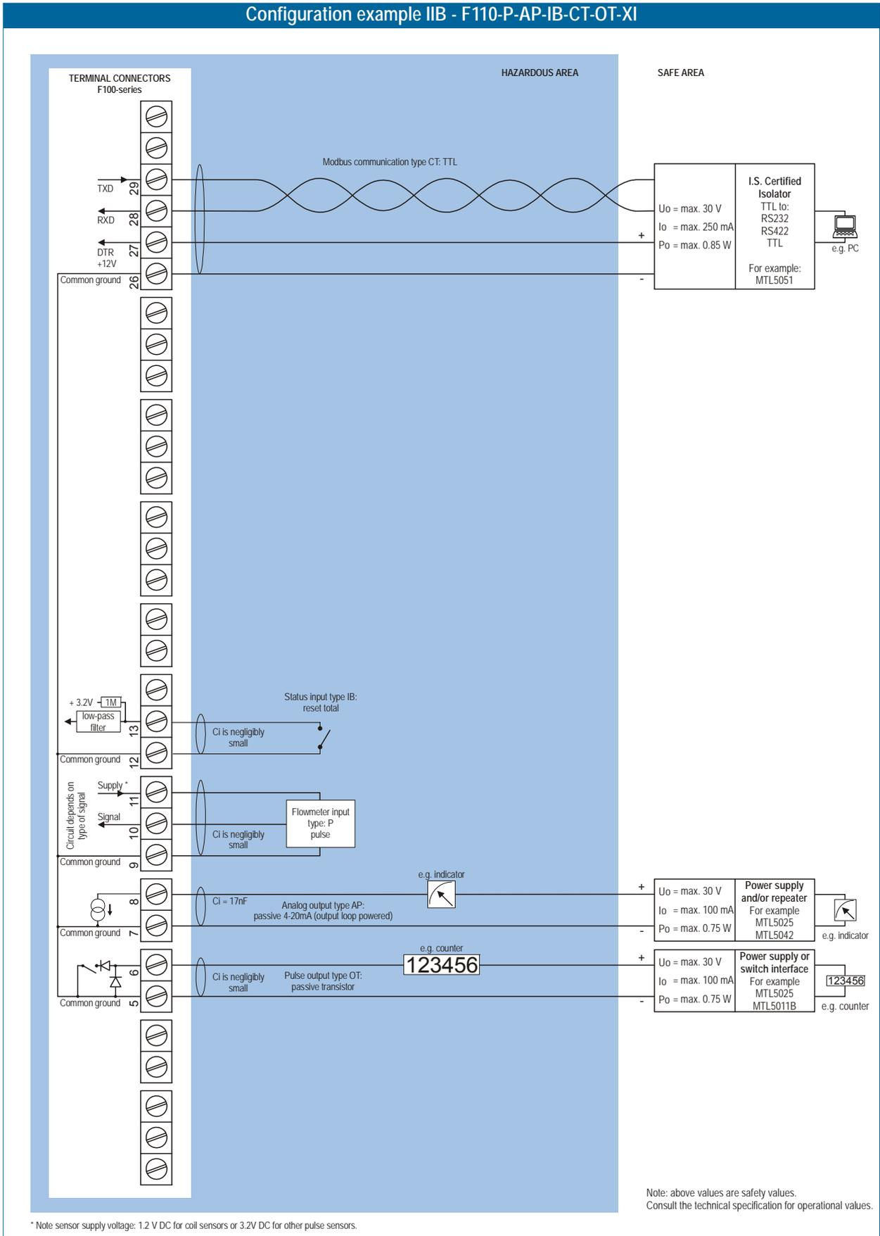
Fig. 14: Configuration example Intrinsically Safe.
