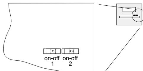
Fig. 13: Switch position voltage selection type PD-XI.
