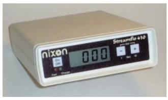
The indicator can read frequency over 1 second or 10 second, can be set to count total pulses, or can be programmed to read velocity directly in cm/sec using data from the individual probes calibration certificate. A 0 to 5 V DC output is available for driving data loggers and chart recorders and this can be programmed to any frequency range.
