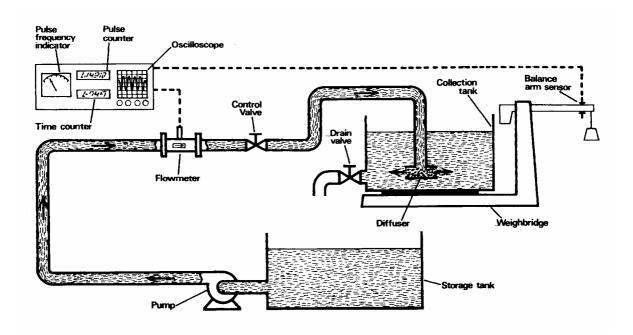
Water is pumped from storage through the test meter, through a manual control valve into a collecting tank mounted upon a standard weighbridge, the vessel having a drain valve for return to storage.At the commencement of a calibration, water iscirculated through the system and allowed to drain whilst the operator regulates the control valve to set up the approximate desired flowrate.
