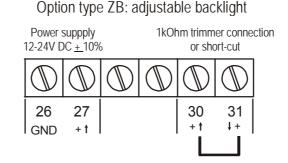
Fig. 11: Overview terminal connectors backlight option.
