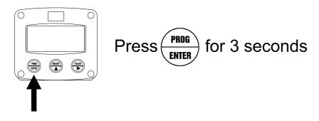
In order to return to the operator level, PROG will have to be pressed for three seconds. Also, when no keys are pressed for 2 minutes, SETUP will be left automatically.
