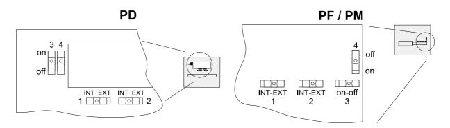
Fig. 8: Switch setting sensor supply voltage.
