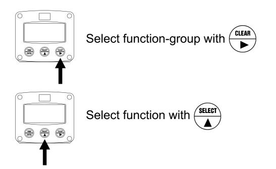
Each function has a unique number, which is displayed below the word "SETUP" at the bottom of the display. The number is a combination of two figures. The first figure indicates the function-group and the second figure the sub-function. Additionally, each function is expressed with a keyword.
