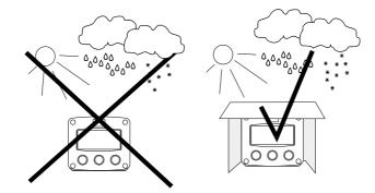
Take the relevant IP classification of the casing into account (see manufactures plate). Even an IP67 (NEMA 4X) casing should NEVER be exposed to strongly varying (weather) conditions. When panel-mounted, the unit is IP65 (NEMA 4)!
