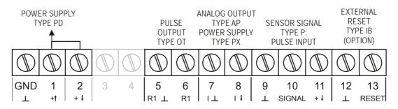
Fig. 12: Overview terminal connectors XI - Intrinsically Safe applications.
