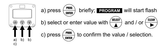
To change a value, use to select the digits and to increase that value. To select a setting, both and can be used. If the new value is invalid, the increase sign or decrease-sign will be displayed while you are programming.
