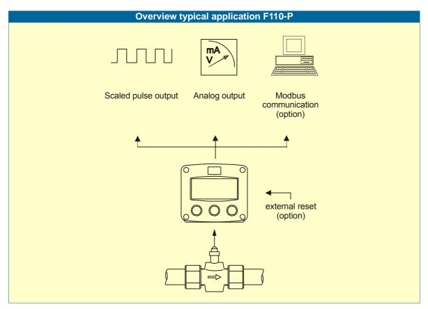
Fig. 1: Typical application for the F110-P.
