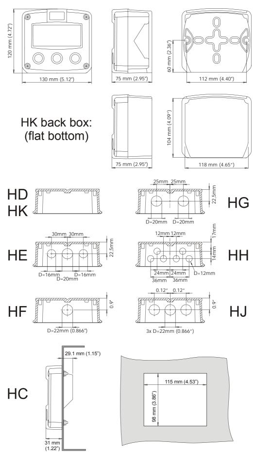
Fig. 6: Dimensions GRP enclosures.
