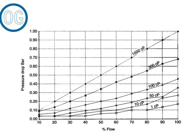
Higher viscosities may be accommodated but the flow range must be reduced e.g. for a viscosity of 2000 cP the maximum flow would be restricted to 80% of the full flow and for 10000 - 40% of full flow.
