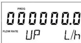
In a CH420L, if during the programming sequence we receive a HART command that must be attended, the local programming will not be valid and all the data previously programmed will be lost. The screen will return to the normal working model and the word PROG will light on the screen, indicating this event. To remove the word PROG from the display, press any of the two PROG push buttons.
