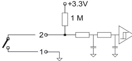
Due to the presence of a filter to avoid the effects of contact bounce, the maximum pulse frequency for the COVOL input is 300 Hz.
