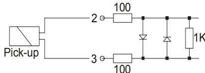
The maximum input frequency is 5000 Hz
