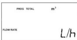
To change the flow rate units, the push button marked with the arrow pointing upwards, must be pushed. To change the totalized volume units, the push button marked with the arrow pointing left pointing upwards, must be pushed.
