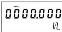
To do this, pushing the push button marked with the arrow pointing upwards, the blinking digit will increase. Once the desired value of the digit is achieved, by pressing the push button marked with the arrow pointing left, the cursor will pass to the next digit to be modified. On the seventh digit, by pressing this push-button the cursor will pass to the first digit on the display.
